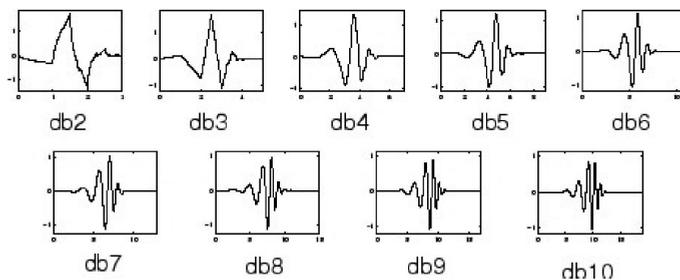
FIGURE 6. Daubechies wavelets ( $N=2,3,\dots$ )
